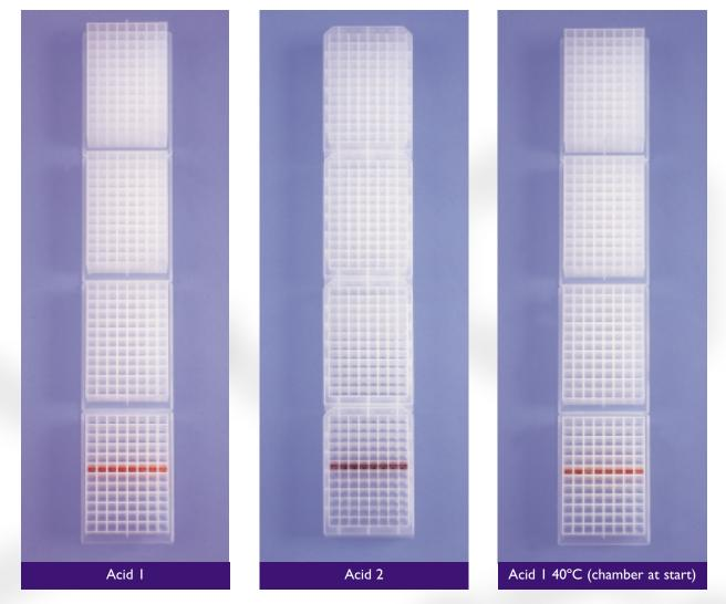
A worse case situation was also evaluated, where the chamber was preheated to 40°C (conditions typically found in a real working situation where the machine had previously been in recent use with a high boiling solvent). Using the same run conditions with Dri-Pure activated there was again complete retention of the samples in their original wells.
