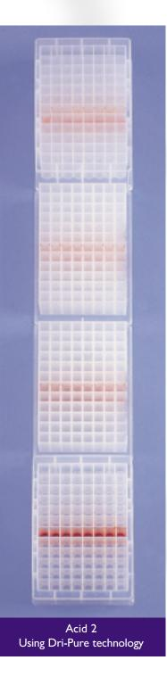
No cross contamination of samples was observed with this solvent mixture, however an interesting effect was seen with the square well plates. Following evaporation of solutions of acid 2, dried sample was present in a discrete band around the inside of each well, approximately **34** of the way up the well. There appeared to be a "corner effect" as each band showed higher travel of the compound in each of the 4 corners.
