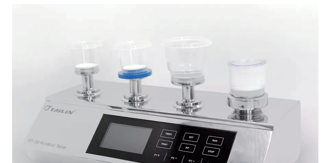
Quick-fit Pump Heads Could Be Heat Sterilized
