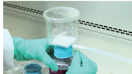
5. After filtering, switch off the vacuum pump, turn the handle 45° to release the pressure and remove the pump tubing.
