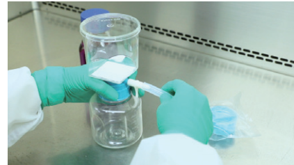
2. Connect the vacuum pump tubing to the hose connector.
