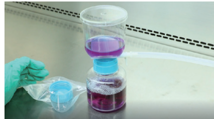
4. Start the vacuum pump for filtration.
